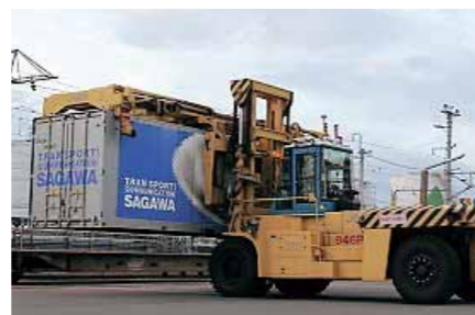
The freight is transferred from Super Rail Cargo to trucks
